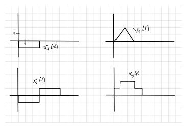
When the input to a linear time-invariant system is given by  $x_1(t)$ , the output is  $y_1(t)$ , see the figure.
